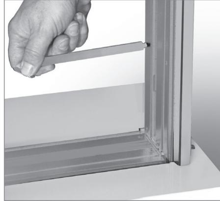
**3.** Suspend the front panel braces in the opening of the inner surface of the shroud element on the left and the right side.
