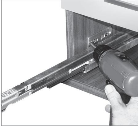
**1.** Fix the full extensions on the right and the left (provide for at least 2 drillings for each strap).
