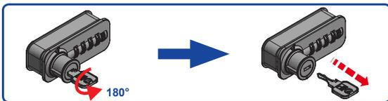
Turn the key 180° to the left. Remove the emergency key.
