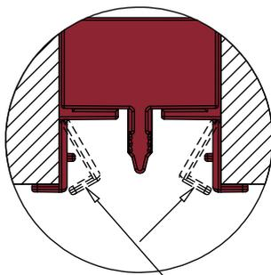
Break the positioning fins of each bearings by folding them inside
