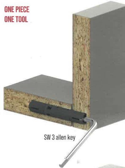
When the key turns CIKO expand in both sides and pull the two panels.
