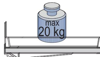
$$+ \text{ (cylinder)} = \Sigma = \text{max } 120 \text{ kg}$$
